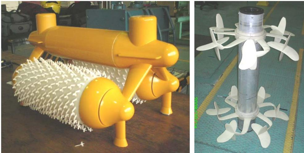
**Figure 1: Model CETUS (left) and CETUS blade test rig (right)**
